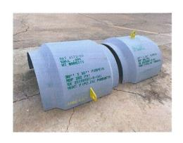
Hunt Pipeline Products manufactures Custom Fabricated Pumpkins to offer a permanent repair over leaking couplings, flanges, valves or screw collars.
